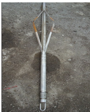
Figure 2. Storage type caliper measuring instrument 图 2. 存储式井径测量仪
