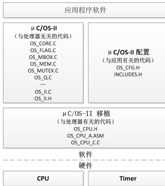
Figure 1. Architecture of \mu C/OS-II software/hardware [4]
