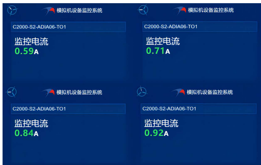
Figure 6. Normal working current of DC motor 图 6. 直流电机正常工作电流
