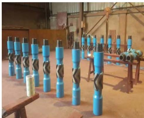
Figure 4. "Short section" debris bed remover
