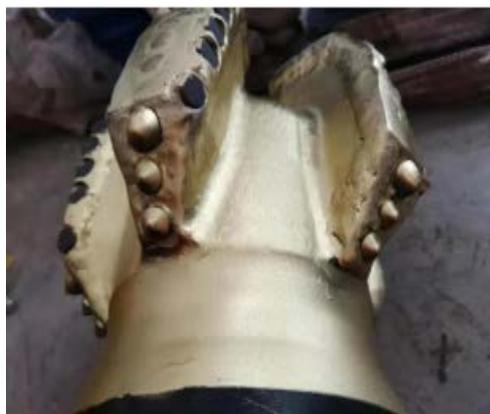
Figure 3. Tapered teeth mounted on the shoulder of the drill
