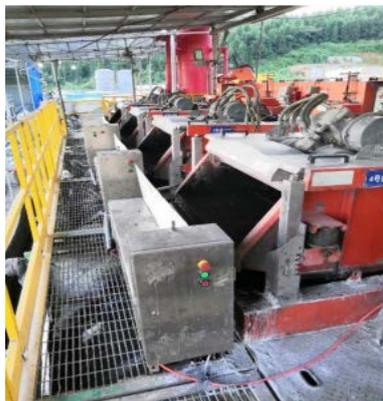
Figure 1. Rock chip flow measurement device
