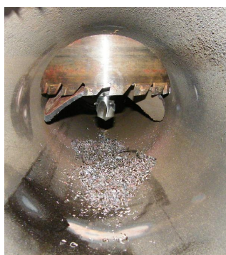
Figure 1. Distribution of iron filings in Hot-tapping test 图 1. 开孔试验的铁屑分布情况
