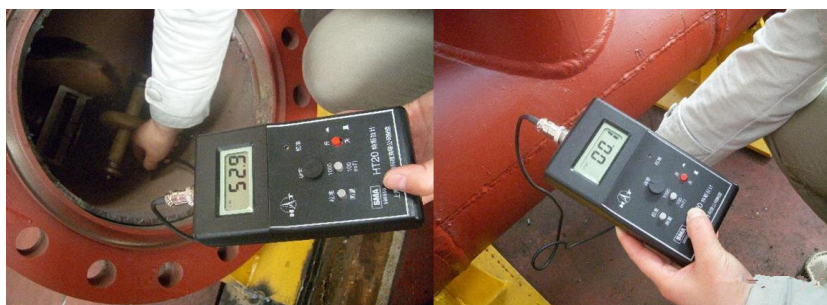
Figure 9. Normal operating condition of the recovery device and residual magnetic measurement after recovery 图 9. 回收装置正常工作状态和回收后的剩磁测量
