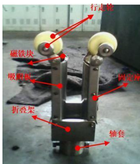
Figure 6. Overall structure of the iron scrap recovery unit 图 6. 铁屑回收装置总体结构
