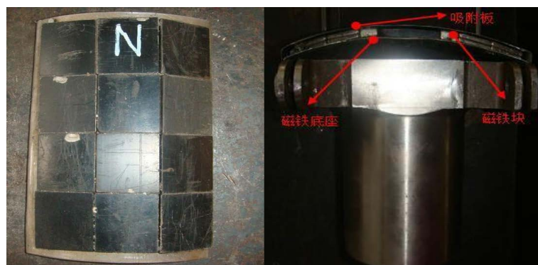
Figure 5. Magnet distribution and the arrangement of the adsorption plate/base 图 5. 磁铁分布及与吸附板/底座的布置情况
