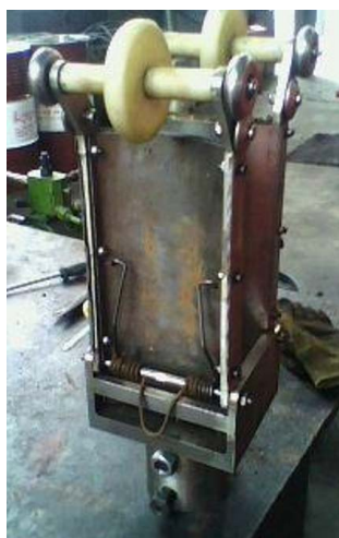
Figure 4. Non-metal and metal combination form of different size wheel
