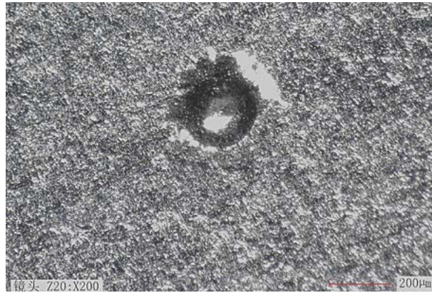
Figure 6. Curve: Speciation of indentation surface under 120 N normal loading
