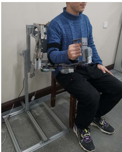
Figure 5. Experimental prototype of neural rehabilitation training robot
