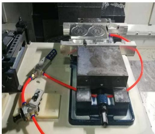
Figure 5. Actual use drawing of the fixture
