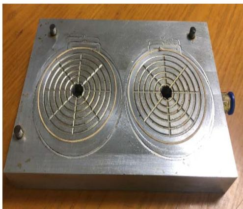
Figure 3. Vacuum chuck
