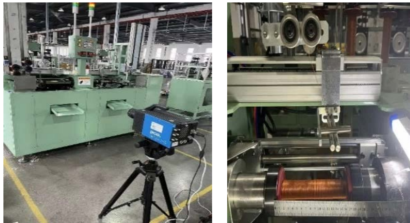
Figure 4. Wire coupling equipment and experimental equipment 图 4. 并丝设备及实验装置
