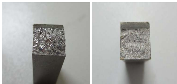
Figure 3. Macrofracture surface of impact test blocks 图 3. 冲击试块宏观断口
