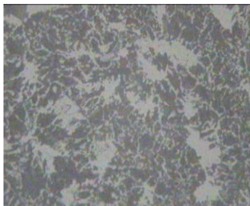
Figure 2. Obvious residue metallographic with abnormal organization × 100
