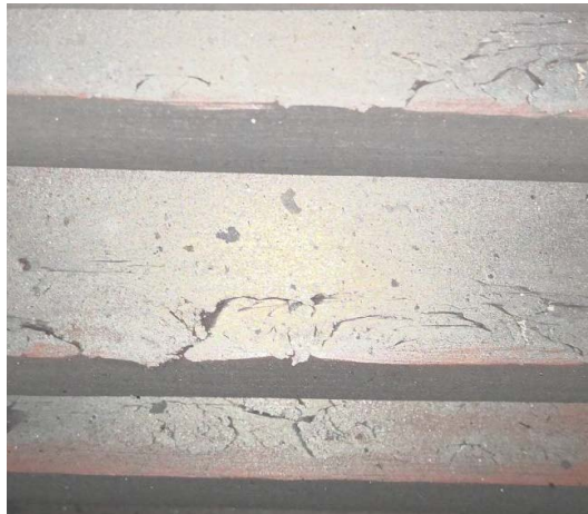
Figure 2. Morphology of irregular crack of 40 mm thickness 45# plate
