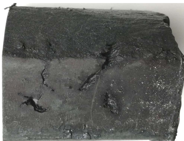
Figure 4. Macro morphology of corner defects of the plate 图 4. 钢板角部缺陷宏观形貌
