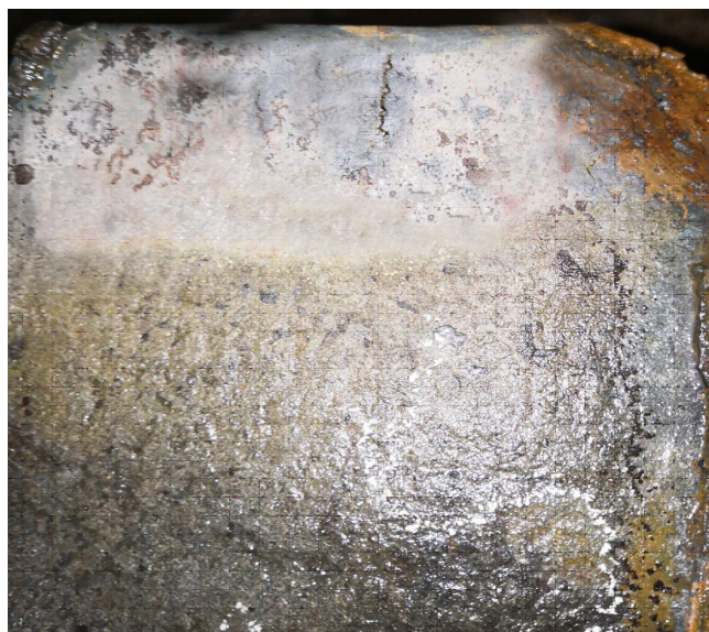
Figure 8. Macro morphology of cracks on longitudinal Plane of 250 mm slab
