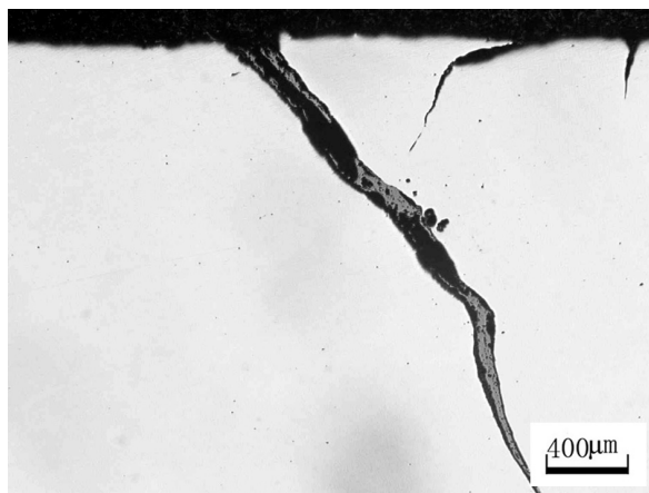
Figure 14. The edge cracks along the original austenite grain boundary of 250 mm slab
