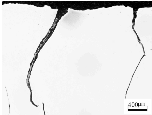
Figure 18. The edge cracks along the original austenite grain boundary of 300 mm slab
