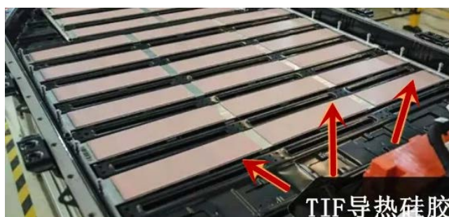
Figure 2. The photo of thermally conductive silica gel loaded into the battery module
