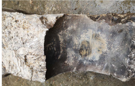
Figure 1. Macroscopic morphology of the fracture interface of Mn18 图 1. Mn18 锤头断裂界面宏观形貌
