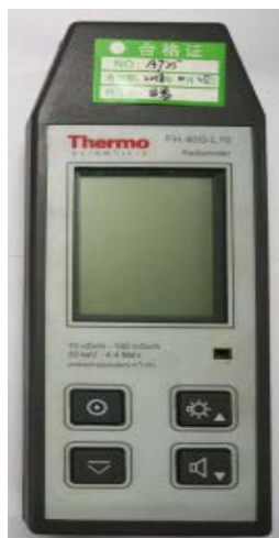
Figure 2. Radiation dose rate meter 图 2. 辐射剂量率测量仪
