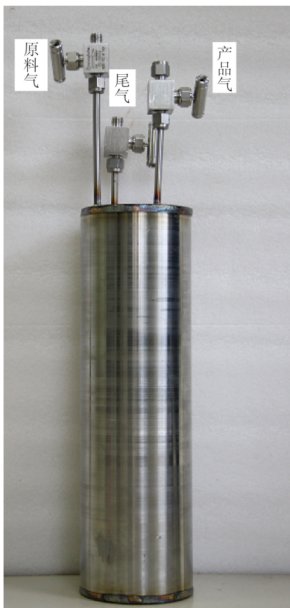
Figure 1. Palladium alloy spiral tube and purification device 图 1. 钯合金螺旋管及净化装置
