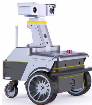
Figure 4. Intelligent patrol robot for substation 图4. 变电站智能巡检机器人
