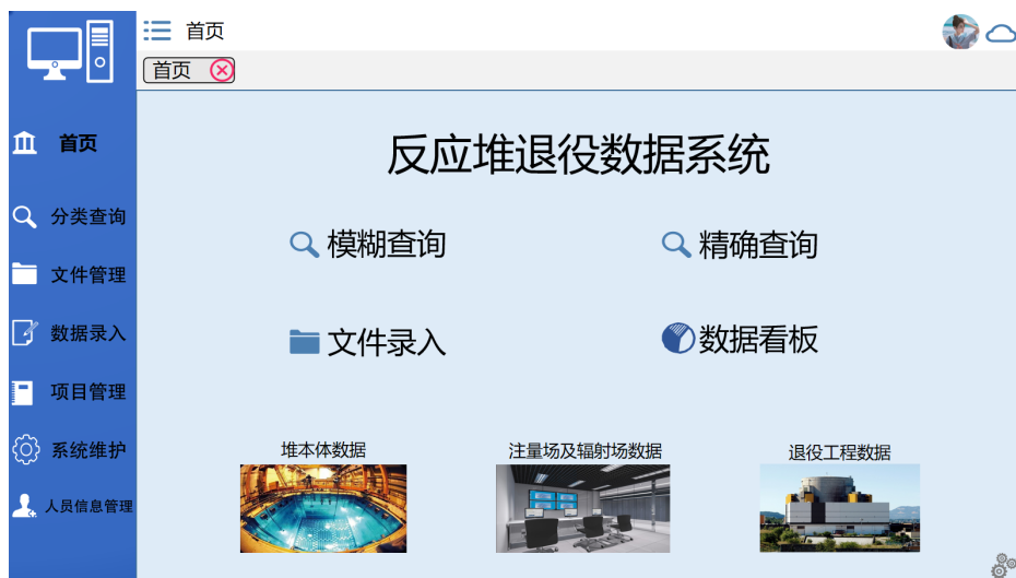
Figure 5. Operation interface diagram of decommissioning data management software of full life cycle 图 5. 全生命周期退役数据管理软件操作界面示意图
