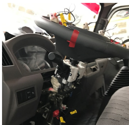
Figure 1. Curve: (a) sensor layout diagram of steering system; (b) the third modes of steering system by hammer test (25.13 Hz)
