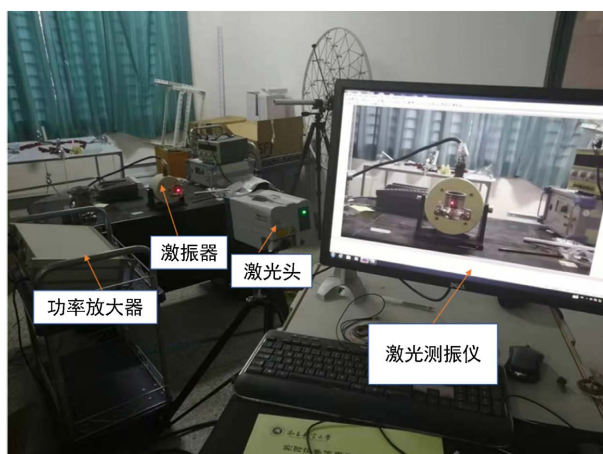
Figure 2. Diagram of a modal measuring device
