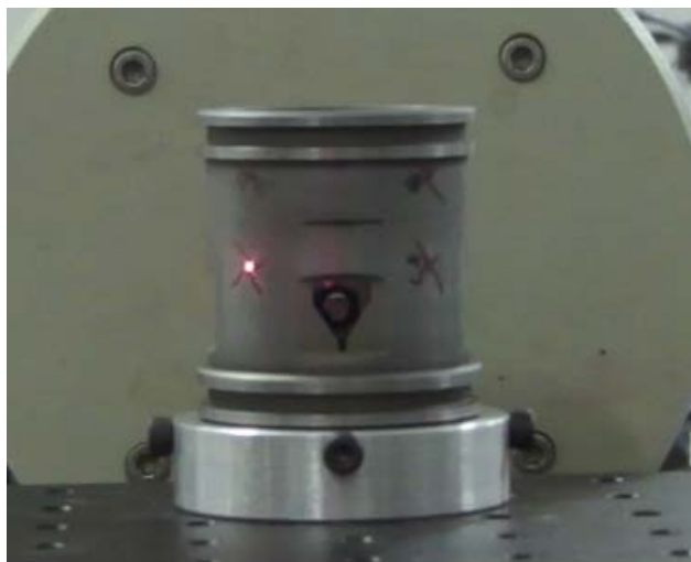
Figure 8. Valve cutting depth 1 mm 图 8. 活门切割深度 1 mm
