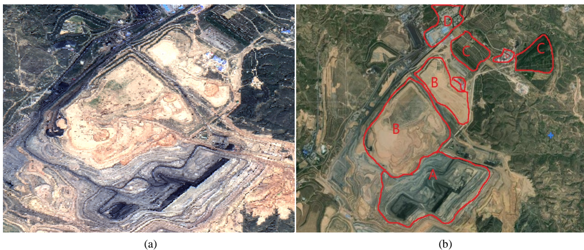
Figure 3. Remote sensing image map and satellite map of Heidaigou open-pit coal mine. (A) Pit; (B) Dump; (C) Reclamation governance; (D) Mine construction
