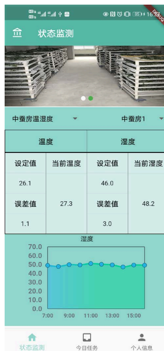
Figure 8. Temperature and humidity monitoring 图 8. 温湿度监测
