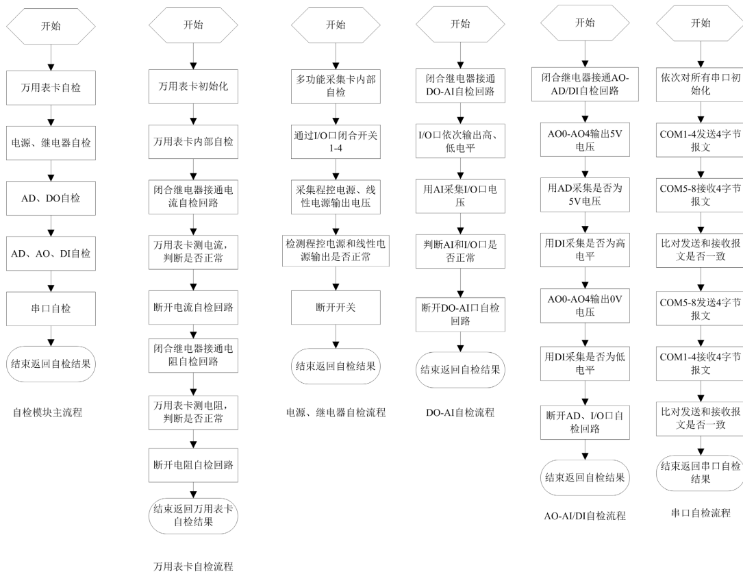
Figure 7. Main flow chart and sub module flow chart of self inspection module
