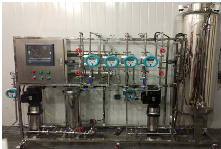
Figure 3. Reverse osmosis membrane test device diagram
