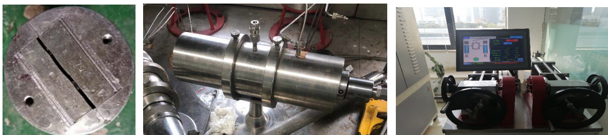
Figure 4. Physical diagram of steel core fracture plate, core gripper, displacement pump and control panel 图 4. 钢制岩心缝板、岩心夹持器和驱替泵及控制面板实物图
