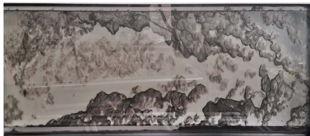
Figure 6. Diagram of experiment on injecting anti channeling plug into flat seams
