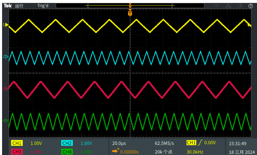
Figure 9. Separation of 30 kHz and 90 kHz triangular wave signals
