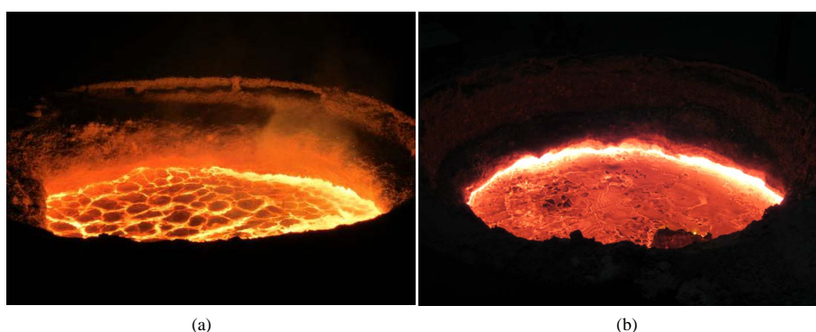
Figure 1. The effect of calcium silicon alloy on slag fluidity; (a) Using calcium silicon alloy; (b) No-using calcium silicon alloy
