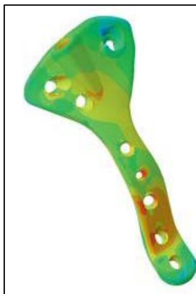
Figure 3. Customized guide plate of new anatomical lock
