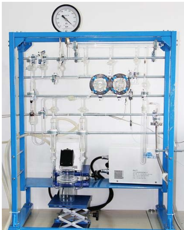
Figure 5. Hydrogen and oxygen collection unit 图 5. 氢气与氧气收集装置
