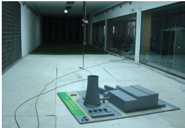
Figure 1. Scene of physical simulation experiment in environmental wind tunnel for the case project 图 1. 案例工程环境风洞物理模拟实验现场
