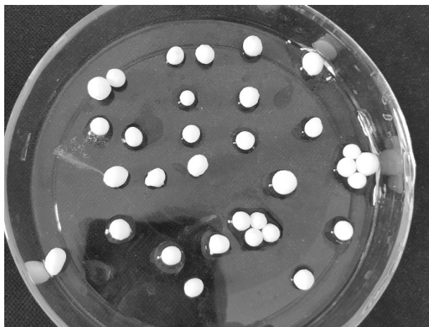
Figure 1. The finished product figure of gel pellets 图 1. PVA 凝胶小球成品图
