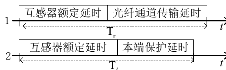
Figure 4. Time delay comparison for the local side MU and remote side MU in data processing and transmission
