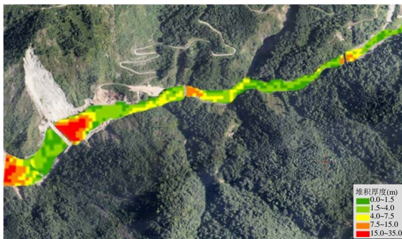
Figure 6. Numerical simulation results of Hongchun gully midstream in the design condition 图 6. 设计工况下红椿沟中游治理工程数值模拟结果
