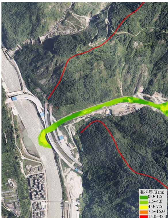
Figure 9. Numerical simulation results of Hongchun gully downstream exceeded the design condition 图 9. 超标工况运行时红椿沟下游治理工程数值模拟结果
