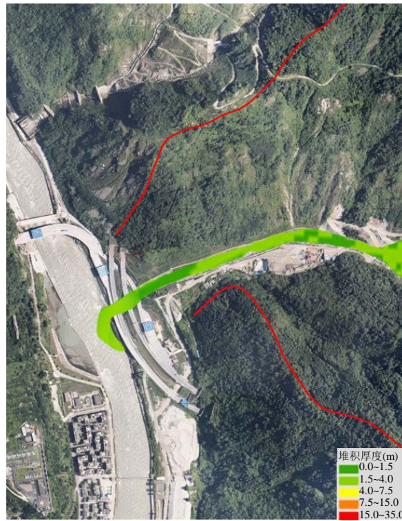
Figure 8. Numerical simulation results of Hongchun gully downstream in the design condition 图 8. 设计工况下红椿沟下游治理工程模拟结果
