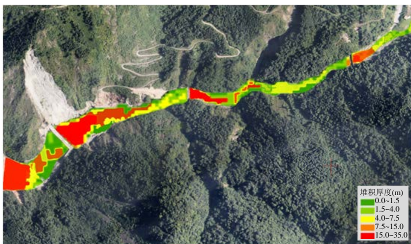
Figure 7. Numerical simulation results of Hongchun gully midstream exceeded the design condition 图 7. 超标工况下红椿沟中游治理工程数值模拟结果
