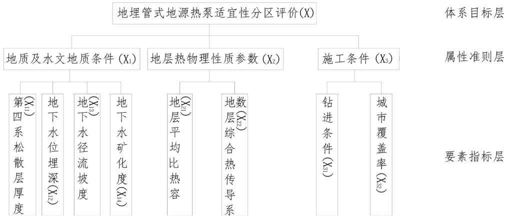
Figure 3. Suitability evaluation system of soil source heat pump 图 3. 土源热泵适宜性评价体系
