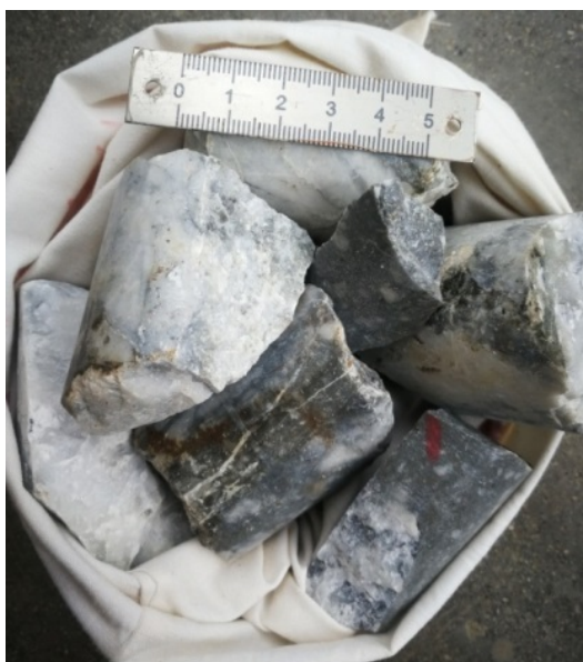
Figure 3. Photo of quartz vein type tungsten mineralized core samples in the contact zone under quartz porphyry dikes in Hetaoping ore concentration area
