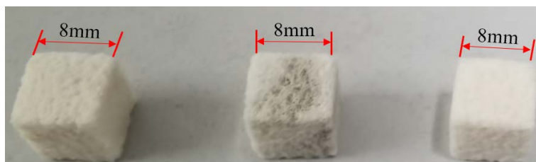
Figure 3. The samples used for MIP measurement, which were taken from the same rock matrix as CR-D
