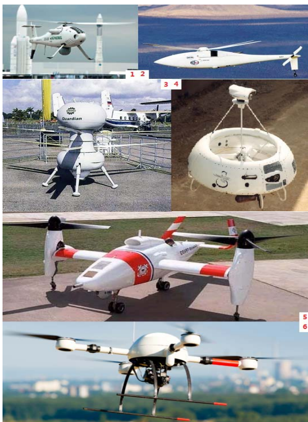
Figure 3. The representation of rotorcraft: (1) S-100; (2) A-160T; (3) CL-327; (4) Cypher; (5) Eagle eye; (6) MD-4
