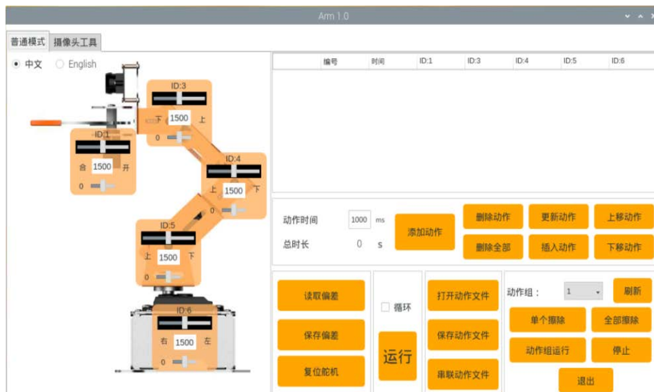
Figure 9. Robot action addition and debugging interface 图 9. 机器人动作添加调试界面
