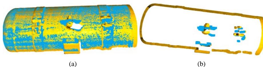
**Figure 10.** Misreport caused by registration deviation of the air cylinder cover plate. (a) ICP registration results; (b) differences points
