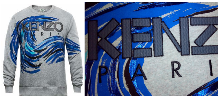
Figure 14. Computer embroidery on silk screen printing 图 14. 丝网印花裁片上做电脑平绣
