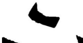
Figure 7. The image after Gaussian filter and binarization
