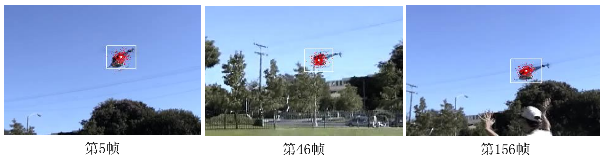
Figure 3. Particle filter tracking results in complex scenes
