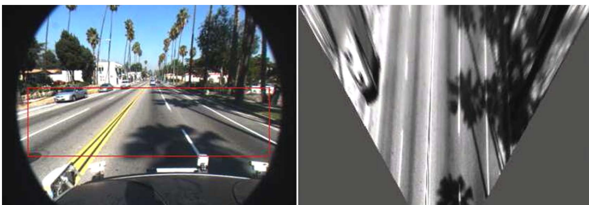
Figure 7. Schematic diagram of inverse perspective projection (Image Credit: Cal tech lane data set)
