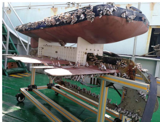
Figure 9. “Sea ray-6000” after 94 days of continuous and reliable operation 图 9. 连续可靠运行 94 天回收后的“海鳐 6000”型波浪滑翔器
