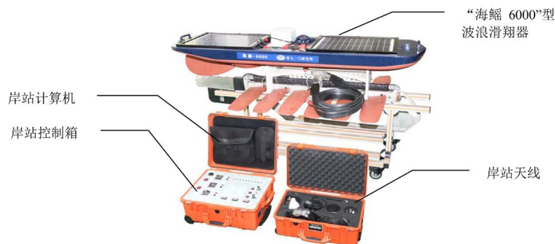
Figure 7. "Sea ray-6000" wave glider and shore station system 图 7. “海鳐-6000”型波浪滑翔器及岸站系统
