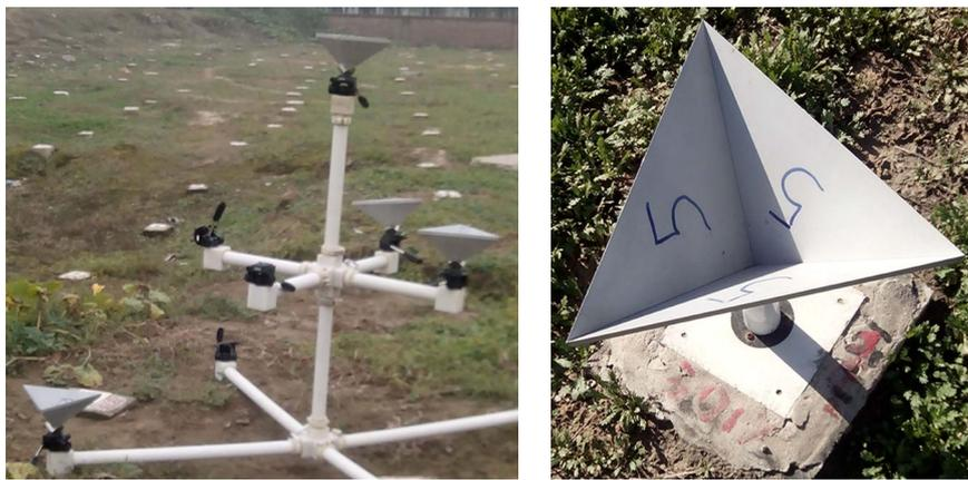
Figure 2. Two main setting mode of corner reflector
