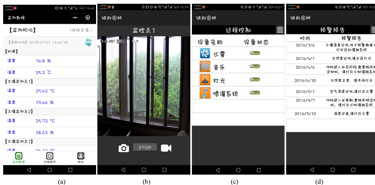
Figure 3. The functional interface of system ((a) Environmental monitoring; (b) Video surveillance; (c) Remote control; (d) Warning notification)
