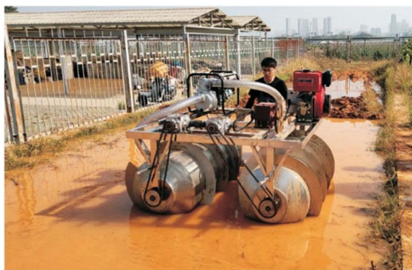
Figure 2. Screw propelled digging machine 图 2. 螺旋推进式挖藕机
