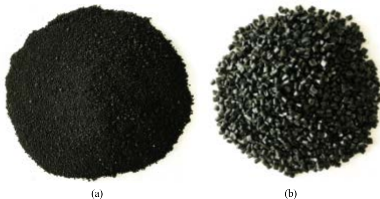
Figure 1. Morphology of two additives (a), waste rubber powder and (b) regenerated PE particles.
