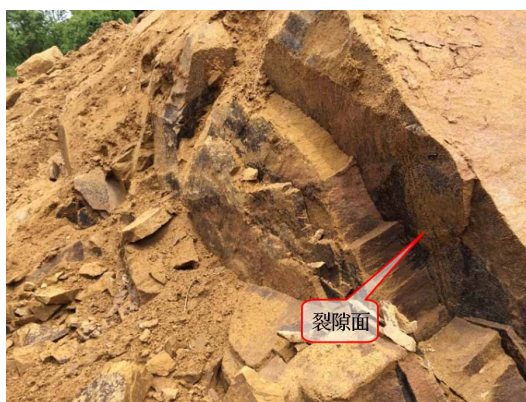
Figure 4. Fracture plane diagram of rock mass
