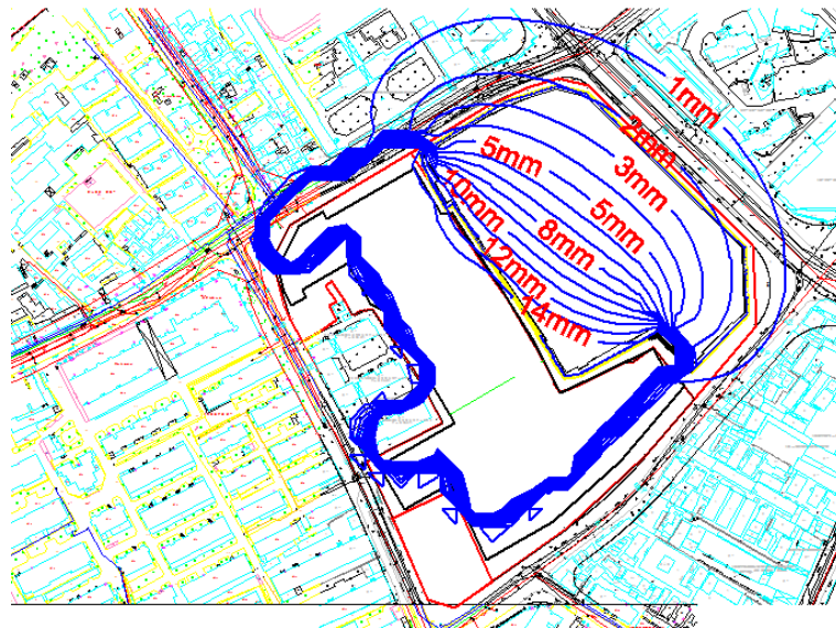
Figure 5. Contour map of ground subsidence around foundation pit caused by decompression and precipitation (unit: mm)
