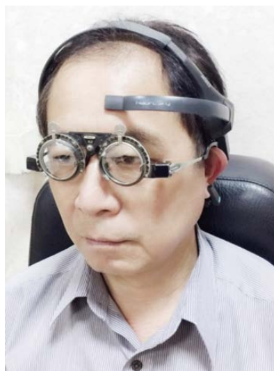
Figure 6. The placement of single pole brain wave capture device and trial frame
